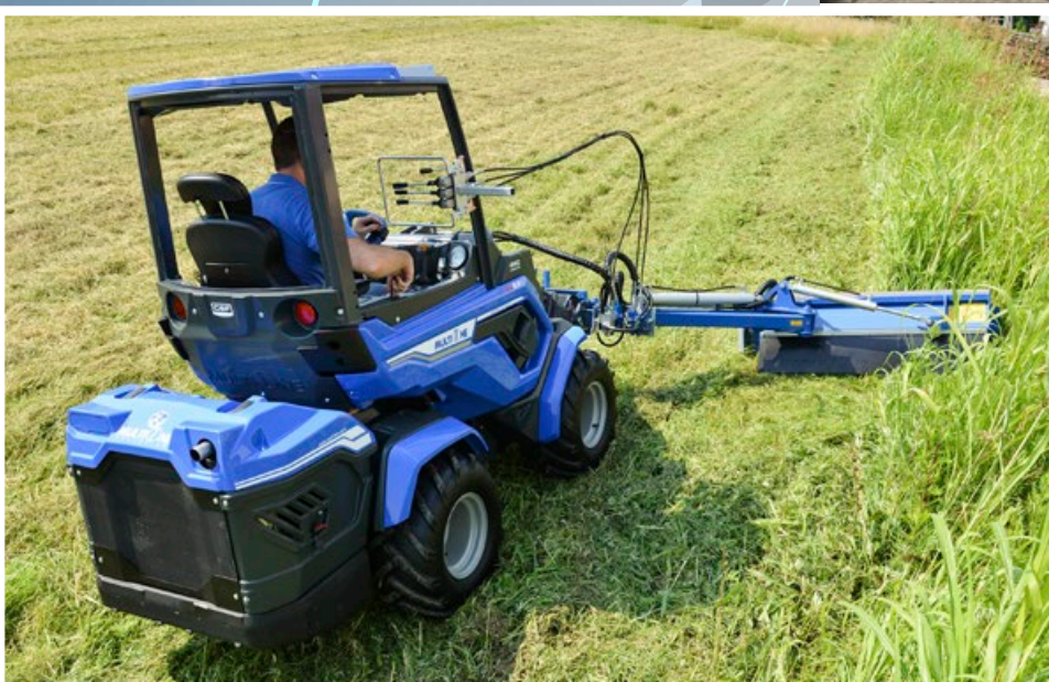
■ Flail Mower With Side Shift
