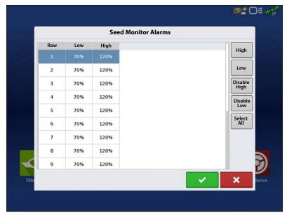
Adjust Seed Tube Monitor Module alarm thresholds. This screen can be accessed in one of two ways:
