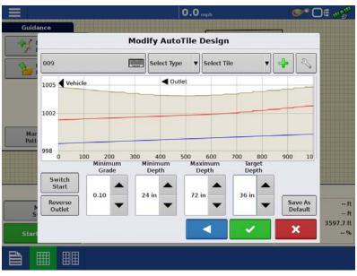
**Maximum Depth**—This is used by AutoTile to know how deep the plow can go. You can either use the maximum depth of the plow or use this to limit the depth you wish the plow to run to lower the pull required if ground conditions are difficult.
