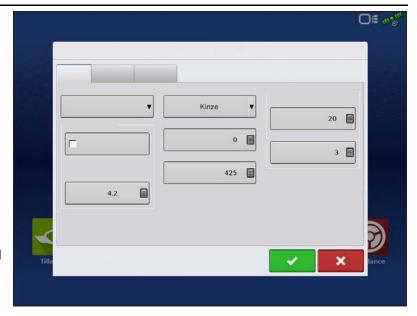
**Hydraulic Pressure to Down Force Conversion**—adjusts system to accurately display changes to hydraulic down force. This setting is row unit specific.
