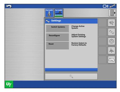
The module must reboot to switch systems. To cancel switching systems, press .
