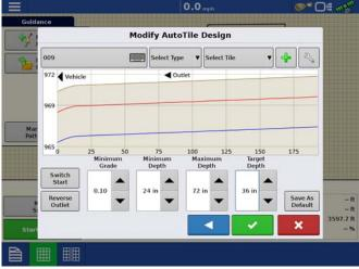
The "Reverse Outlet" button changes which end the outlet is on. The outlet end is the end of the path towards which the water drains. There is no effect on the ground profile, which remains unchanged. The difference appears in the shallowest and deepest installation profiles, which now are designed to drain in the opposite direction.
