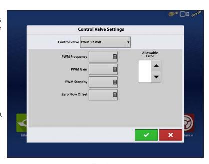
cause the product control system to not properly control low rates or shut off. Default Value is 30. See the PWM valve manufacturer information for recommended settings.
