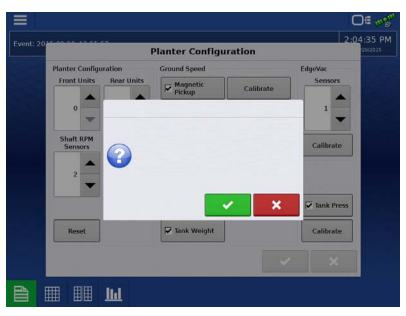
2. **Detect individual row units**—Plug in each physical sensor plug into the Muxbus wiring harness on the planter (from left to right). Follow the on-screen instructions.
