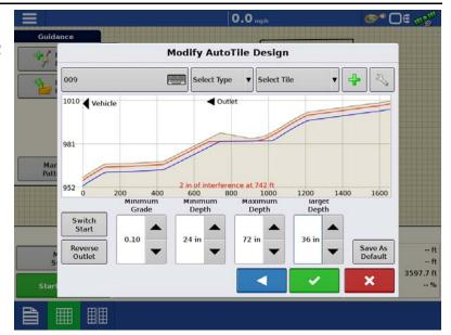
Increase the "Maximum Depth" to 75 in. to create a solution. The shallowest solution requires us to start at least 2.2' deep. Start at this depth or any depth greater.
