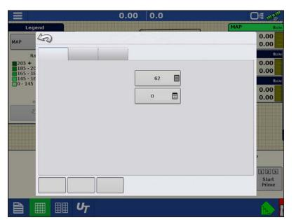
**In-Field Calibration**—Press the In-Field Calibration button to perform an automated routine to adjust the calibration number for the selected metering circuit. This calibration is performed if there is a difference between the amount of product logged as compared to what was actually applied. For more information, see "In-Field Calibration Procedure" on page 451.
