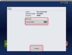
**8.** On the iPad, open the AgFiniti Mobile app. Once the AgFiniti Mobile is open, it will automatically attempt to connect to the InCommand display.
