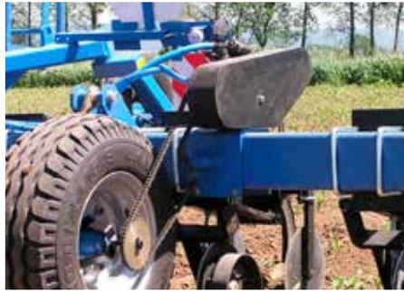
Simple dose setting in the range of 70 to 170 l.ha<sup>-1</sup>. The dosing pump is powered by the gauge wheel via a sprocket gear. Changing the sprocket changes the fertilizer dose.
