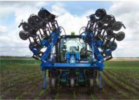
The frame consists of a robust profile with mounted hydraulics for easy tilting between working and transport positions. The transport position gives the operator a clear view to ensure safe transport on public roads.
