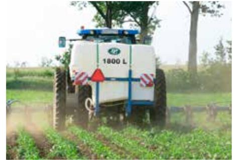
Big liquid fertilizer tanks – 1800 l for PPL 12 front and 1400 l for PPL8.6 – guarantee high machine performance. A clean water tank enables easy flushing of the distribution system and filters at the end of the shift.
