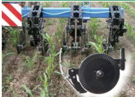
Application units with coulters are designed for soil protecting techniques where there are extensive organic residues on the soil surface. The protective function of mulch is not affected and they prevent the clogging of working tools.
