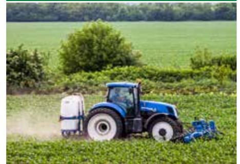
High operating speeds of up to 12–16 km.h<sup>-1</sup> allow a daily PPL-12 performance of up to 80 ha, with low fuel consumption.
