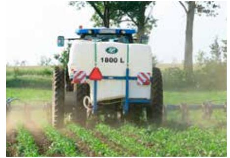
Big liquid fertilizer tanks – 1800 l for PPL 12 front and 1400 l for PPL8.6 – guarantee high machine performance. A clean water tank enables easy flushing of the distribution system and filters at the end of the shift.
