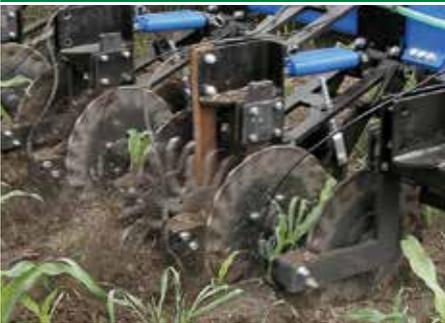
Star cultivating wheels with fertilizer application discs for breaking the soil crust work well in light compaction conditions when operating on medium soils.
