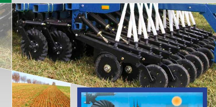
This seeding machine may also be used for improved or additional crop seeding in the case of irregular germination or growth damage. The seeding structure is also designed for leguminous and oil plant seeding.
