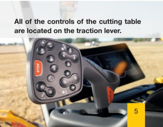
**All of the controls of the cutting table are located on the traction lever.**
