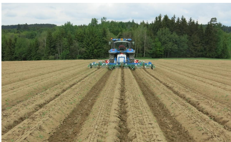
Fig. 8: Application of fertilizers before growth into the root zone of plants by machine VARIOR 500.
