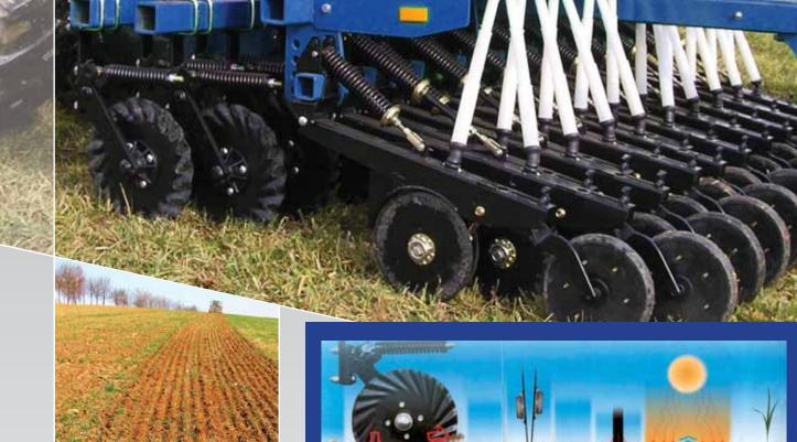
This seeding machine may also be used for improved or additional crop seeding in the case of irregular germination or growth damage. The seeding structure is also designed for leguminous and oil plant seeding.
