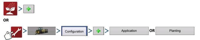
WARNING! When setting up a Configuration for the Serial Application Rate module, on the Application Channels step of the Implement Wizard, a controller may default in this screen based on the displays Load-and-Go feature. DO NOT accept this controller for the configuration. Delete this controller by highlighting it and pressing Remove. Then create a new Liquid/Granular Application controller manually.
