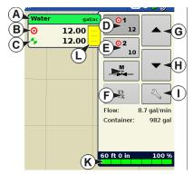
NOTE!: In some conditions, the Actual Rate may increment slower than the Target Rate, or its numeric values may vary before matching the Target Rate.
