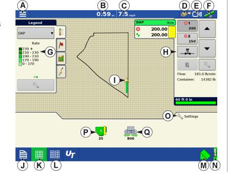
view shows the Rate butons, Manual Valve Control button, Prescription button, Rate Increase and Decrease arrows, and the Rate Setup button.
