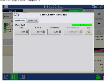
**Minimum Flow** — (Used for DirectCommand Liquid Applications only). This setting is used to
