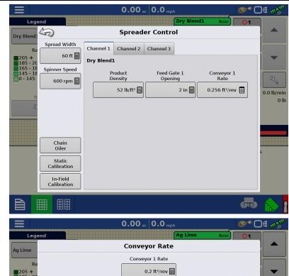
The **Conveyor Rate** button opens a setup screen where the conveyor rate can be input, and a table of previously applied products and conveyor rates is shown.
