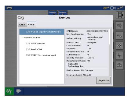
Pressing the Diagnostics button on the Devices screen brings up the ISO Node Diagnostics screen which shows the following information.
