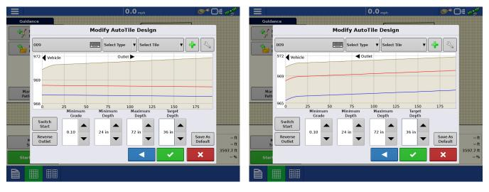
The "Reverse Outlet" button changes which end the outlet is on. The outlet end is the end of the path towards which the water drains. There is no effect on the ground profile, which remains unchanged. The difference appears in the shallowest and deepest installation profiles, which now are designed to drain in the opposite direction.
