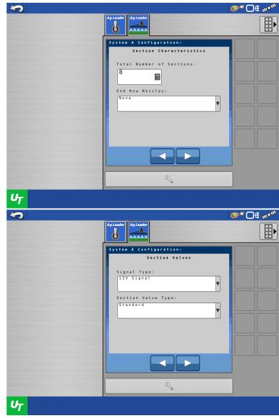
4. Edit the signal type or section valve type if necessary, press
