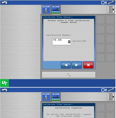
3. The calibration is complete and new calibration number sound be displayed.
