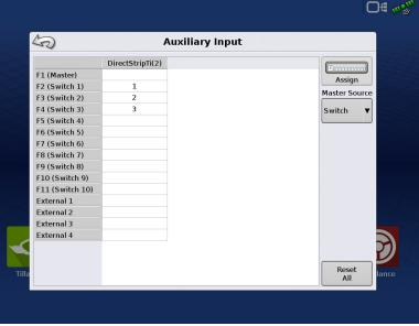
3. Select appropriate function(s) (bins for this operation) to be assign to the desired switch. Chain icons within each function will "link" once pressed to indicate they are assigned. If a function has a "broken link" then it is not assigned. If a switch has a "X" then it is not assigned to a function. Press
