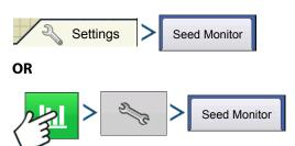
The Planter Options screen adjusts Seed Tube Monitor Module alarm thresholds, Gain, and Advanced Seed Monitoring alarm thresholds. The screen also has access to module Diagnostics.
