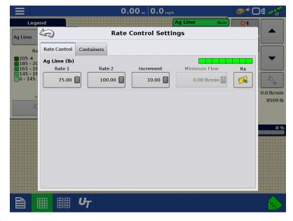
maintain a consistent spray pattern. The display will not allow flow to drop below the entered setting. Set to flow at the lowest operating pressure for the selected spray tips with all sections on. When spraying with one or more boom sections off, the system automatically reduces the minimum flow setting according to the reduced spray width. To adjust this setting, press and enter the desired numeric value.
