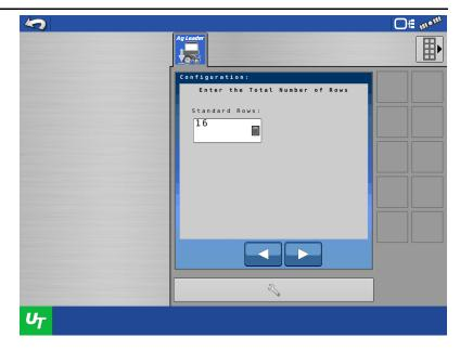
**3.** Enter the number of control channels. This will be equivalent to the number of valve sections. Typically this will range from 3 to 8 total sections.
