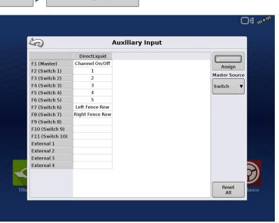
3. Select appropriate function(s) (boom sections for this operation) to assign to the desired switch. Chain icons within each function will "link" once pressed to indicate they are assigned. If a function has a "broken link" then it is not assigned. If a switch has a "X" then it is not assigned to a
