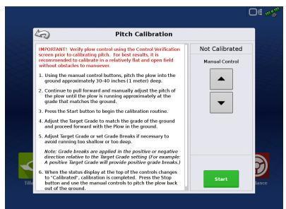
Pitch calibration number determines sensor reading for level installation. Plow status will read "Not Calibrated" until Pitch calibration is ran. Only after having followed those instructions will you need to adjust this pitch zero number.
