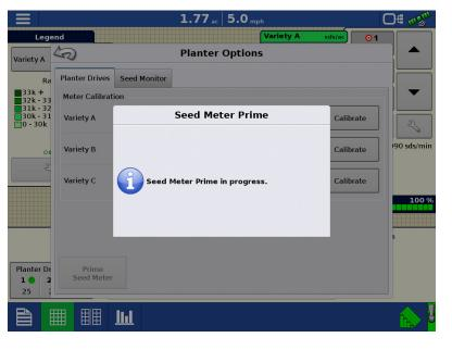
A message displays, stating "Seed Meter Prime in Progress." While this message displays, the seed meter will turn one (and only one) revolution automatically. When complete, return to the Planter Options screen.
