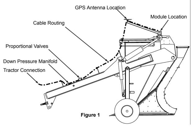
Locate cable PN 4003415. This will be mounted on the plow, with the single round cable connector at the hitch. There are 2 weather pack connectors that will connect to the Proportional valve. If you cannot route the cables to make these ends work, extensions can be ordered by your dealer to make the connections. Route the cable as shown below to ensure that moving parts do not pinch cables, extensions, or adapters.
