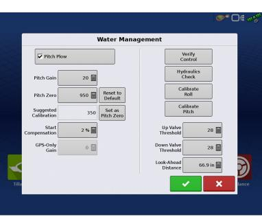
commands (for example if the UP button makes the plow go down) change the Valve Polarity setting and try again.
