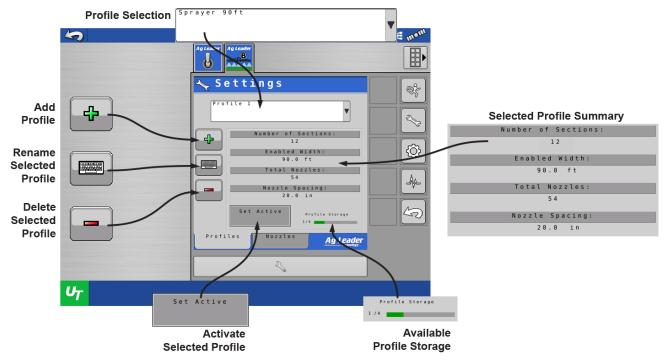
Creating machine profiles is useful when there is more than one possible configuration of the same machine. For example, if a user sprays with the entire 120ft boom of their sprayer on one field. On the next field they fold in their extensions to only spray using 90ft of the swath width. Creating a profile for each scenario will prevent accidental activation of sections that are folded causing over application. Each system can have up to 4 profiles saved.
