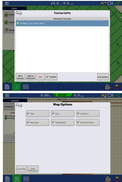
If you have RTK GPS reception, you are allowed to collect an elevation survey. This will allow you to collect the Latitude/Longitude and elevation values as you traverse the field.
