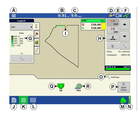
During DirectCommand Run Time operations, the Product Tab(s) are shown in the upper right-hand side of the Map screen. Press the Product Tab(s), and an extended view shows the Rate butons, Manual Valve Control button, Prescription button, Rate Increase and Decrease arrows, and the Rate Setup button.
