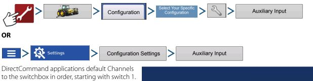
DirectCommand applications default Channels to the switchbox in order, starting with switch 1. From the Auxiliary Input screen, the operator can customize the switches to certain channels, if desired.
