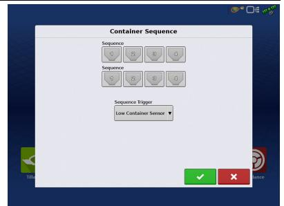
5. Use Sequence Trigger drop-down menu to select container advanced trigger method.
