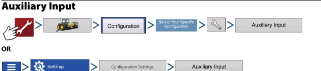
DirectCommand applications default boom sections to the switchbox in order, starting with switch 1. From the Auxiliary Input screen, the operator can customize the switches to the boom sections, if desired.
