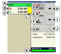
**Rate 1 and Rate 2** — The Rate 1 and Rate 2 settings represent preset application rates that allow operators to quickly change between desired target rates for each individual product.
