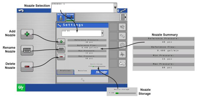
Creating nozzles is required for pressure based control, pressure fall-back, and droplet size monitoring. A nozzle's specifications are needed to achieve each feature.
