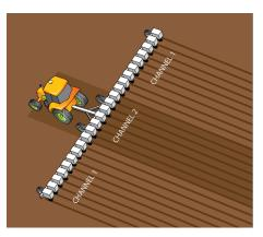
The system can be split between two channels to allow the down force to be adjusted separately on the planter wings and center section, where soil compaction is more likely to occur.
