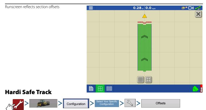
When using Hardi ISOBUS, Implement Modeling can be set to Hardi SafeTrack. This allows display to accurately calculate path of sprayer.
