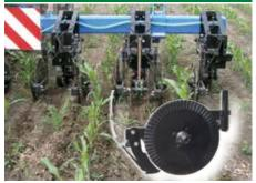
Application units with coulters are designed for soil protecting techniques where there are extensive organic residues on the soil surface. The protective function of mulch is not affected and they prevent the clogging of working tools.
