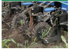
Star cultivating wheels with fertilizer application discs for breaking the soil crust work well in light compaction conditions when operating on medium soils.
