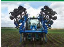
The frame consists of a robust profile with mounted hydraulics for easy tilting between working and transport positions. The transport position gives the operator a clear view to ensure safe transport on public roads.
