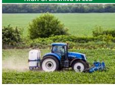
High operating speeds of up to  $12-16 \text{ km.h}^{-1}$  allow a daily PPL-12 performance of up to 80 ha, with low fuel consumption.
